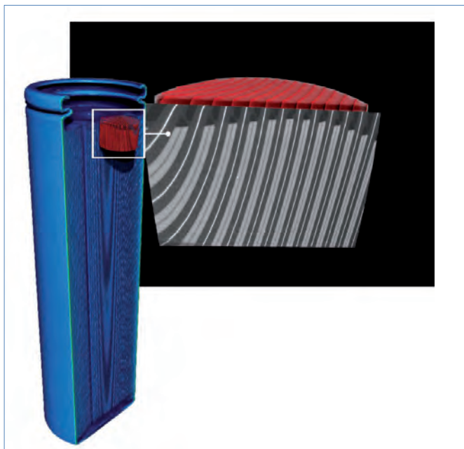
Image 4: Flat panel imaging of a cylindrical 21700 battery shows full cell visualization and a magnified high-resolution view of a selected region, highlighting the internal layered structure for detailed, non-destructive characterization.
