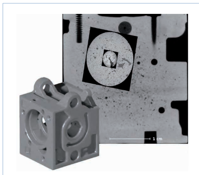
Image 3: 3D rendering of an aluminum block with reconstructed slice overlays illustrating seamless multi-scale zooming capabilities for rapidly locating regions of interest in a 30 mm cube sample.
