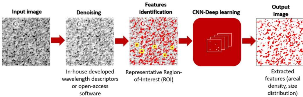
Illustration of the methodology using CNN detectors applied to an inverse WBDF image presenting dots-shaped dislocation loops formed in a Co-free HEA irradiated with 2 MeV Fe ions at liquid nitrogen temperature.
