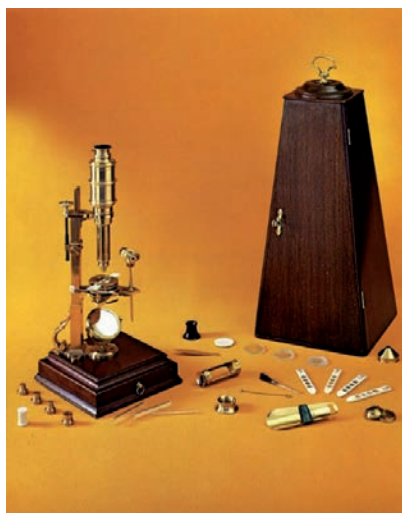
Figure 1. Compound microscope of ~ 1750, attributed to John Cuff
