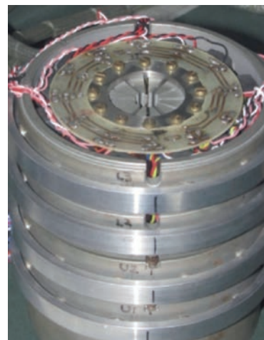
"The central part of the first STEM Cs corrector that improved the resolution of the microscope it was built into, with multipole stages containing strong quadrupoles and octupoles, and 96 auxiliary coils for nulling parasitic aberrations. Corrector Ø-12 cm." - Reprint of Figure 2 from Ondrej Krivanek's autobiography: http://kavliprize.org/prizes-and-laureates/prizes/2020-kavli-prize-nanoscience
