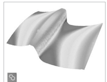
Fig. 3 : 3D topography for the same dental implant using confocal fusion technique
