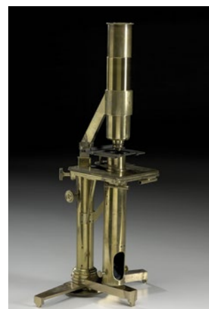
Figure 7: (right) An original Valentine microscope as built by Ross (1831) in its compound version. Valentine's own copy. Do notice the long tube underneath carrying the mirror and meant to reduce false light. Courtesy: the Tasmanian Museum and Art Gallery.
