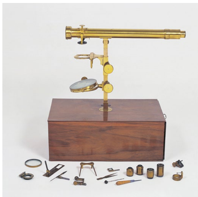
Figure 2: A catadioptric microscope built by Amici with its accessories. Courtesy: Museo Galileo, Florence (inv. N°3171; ©Franca Principe).
