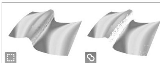
Fig. 2 : 3D topography for a dental implant respectively using Focus Variation and Confocal techniques
