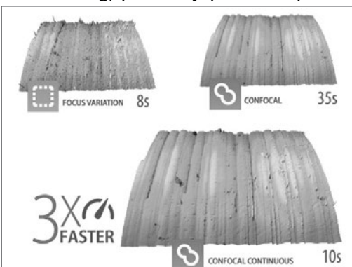
Fig. 1 : Speed comparison: Confocal Continuous technique three time faster than Focus Variation and Confocal modes
