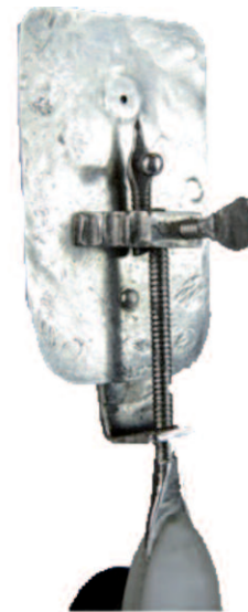
Fig.6 The newly recovered Leeuwenhoek microscope with a blown lens in a silver setting (collection: Bert Degenaar).
