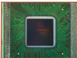
Global Ultra Thinning (to less than 5 microns)
