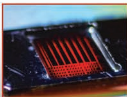
Site-Specific Ultra Thinning (to less than 5 microns)
