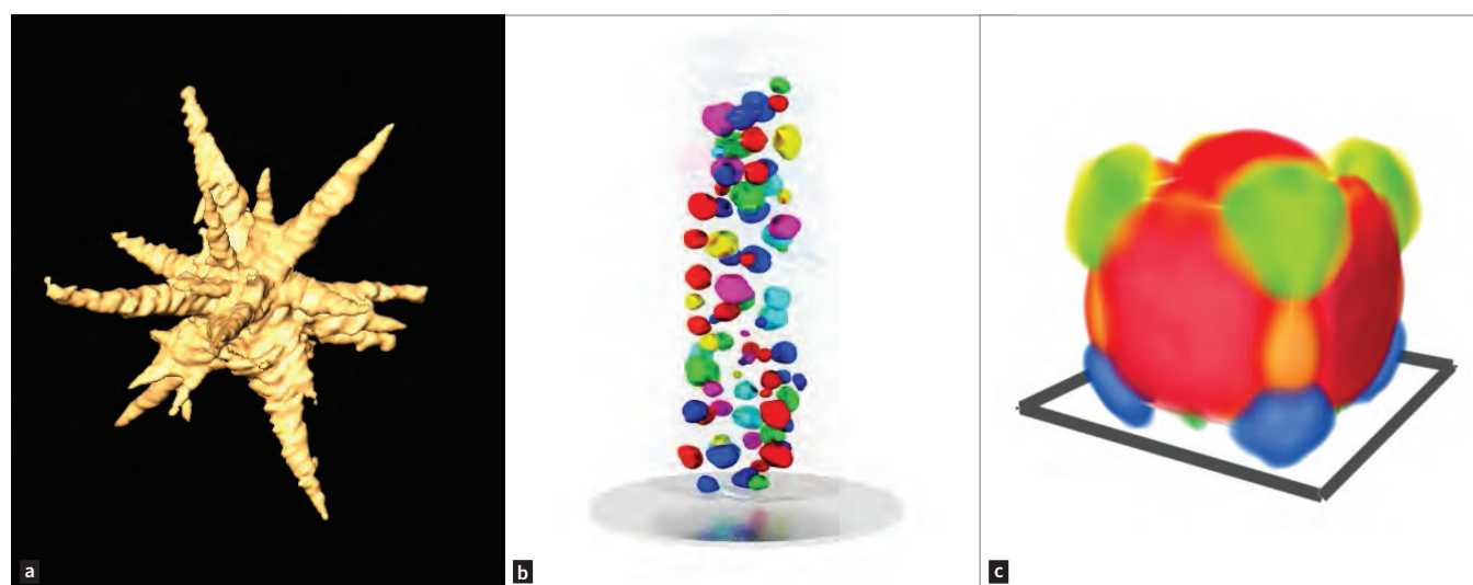
Figure 1. 3D tomographic reconstructions of (a) a CdTe ‘multipod’ using HAADF-STEM imaging; (b) precipitates in a Ni base superalloy using STEM-EDX tomography [3] ; (c) localized surface plasmons on the surface of a Ni nanocube using low loss EELS tomography [5] .
