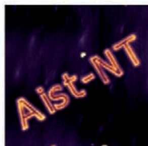
Lithography on GaAs film 3x3 μm
