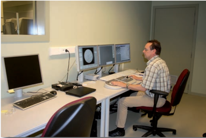
Remote control of the Qu-Ant-EM microscope from the separated control room
