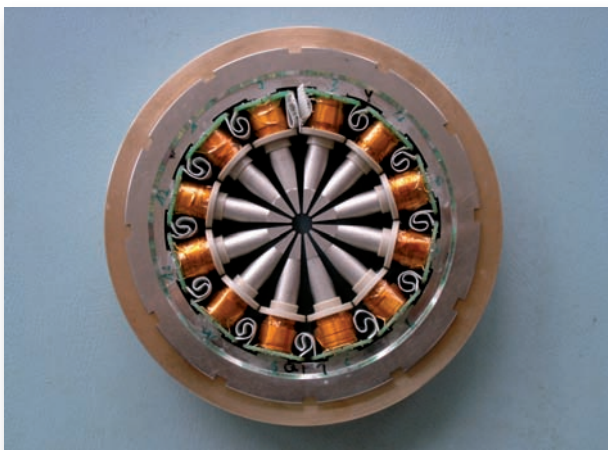
"Darmstadt-Corrector": the image shows the longitudinal cross section through its final version, with the dodecapole lens in the middle, as developed and tested by Max Haider in his diploma thesis.
