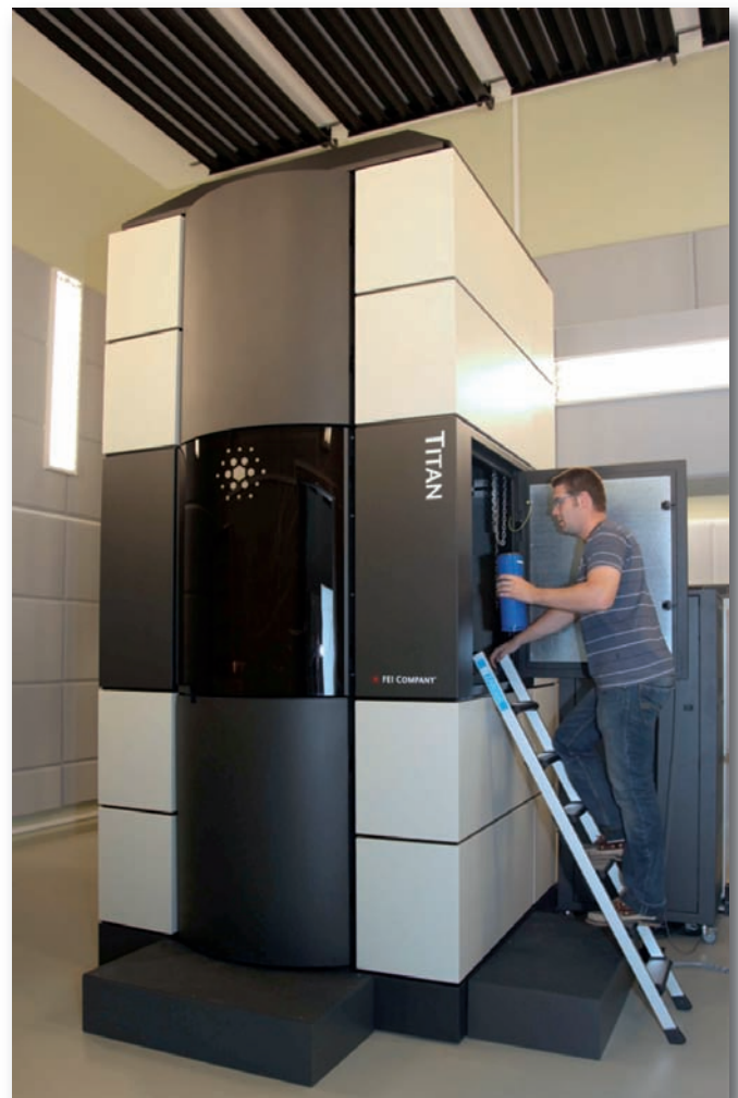
The Qu-Ant-EM microscope in its cube enclosure and dedicated environmentally shielded room
