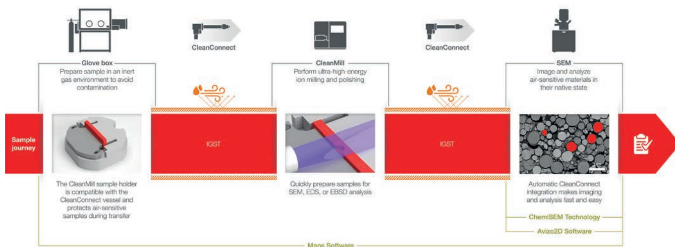
Figure 3 Inert gas workflow for nanoscale analysis using Thermo Scientific CleanMill and SEM
