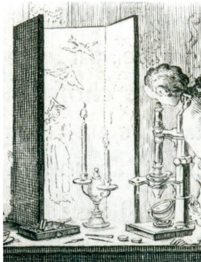
Figure 4 : Cut-out from an engraving by François Antoine Aveline. We see Daubenton using a Cuff-type microscope to study a preparation. Two candles serve as light-source, a gilded(?) Chinese draught-screen as a primary mirror. Source: Buffon, Histoire naturelle [...], volume II (1749), p.1. Courtesy: Bibliothèque Nationale de France, Paris.
