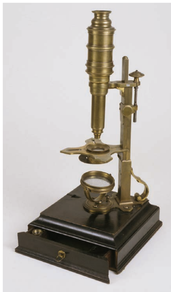
Figure 3 : Cuff microscope (ca.1745). The cross-like object table features a 'Lieberkühn'-mirror for extra on-top illumination and two slots, the one for a condenser lens, the other for objects e.g. on top of a needle. The mainbody is fixed to a compound pillar, allowing for crude and fine tuning. Courtesy: Whipple Museum, Cambridge.
