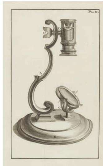
Figure 5 : The scroll-mounted screw-barrel microscope according to Henry Baker. From the Dutch translation (1744) of his work The microscope made easy [...] Courtesy: University Library Groningen.
