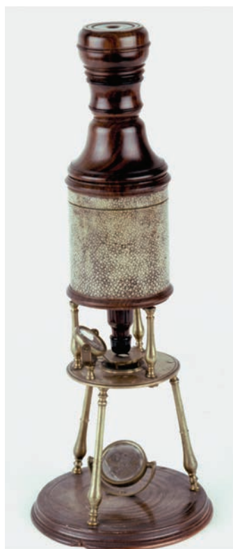
Figure 2 : Culpeper microscope (ca.1730). The eyepiece (ocular plus field-lens) may be shifted in the mainbody depending on the particular objective used. Do notice the extra lens at the object table and the sub-stage spherical (!) mirror. In the present state it is ready to be used for the study of slide-sticks, samples between muscovy-glass in ivory holders. Courtesy: Whipple Museum, Cambridge.
