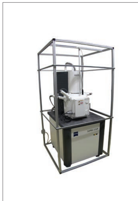
→ Active magnetic field cancelling system - example of local isolation for SEM
